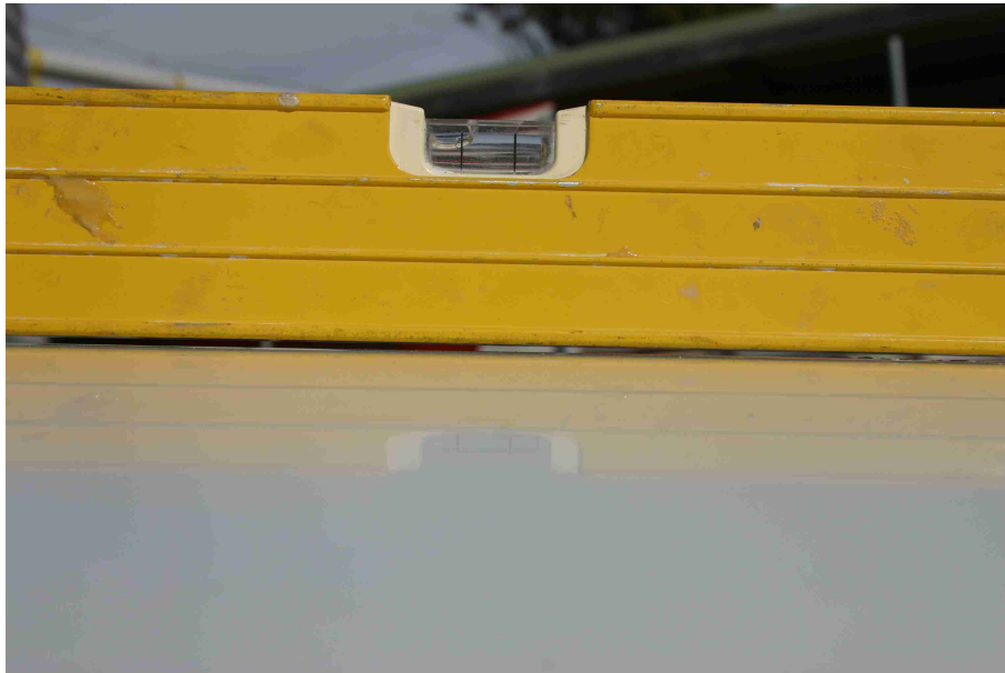
Bottom section of the 49er master plug : 3mm hollow
