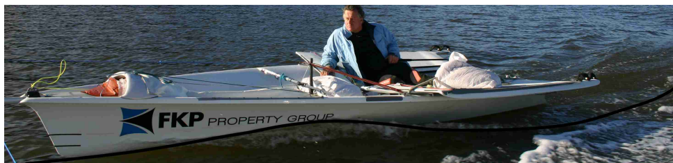
Over hull speed, the second crest is aft of the transom
